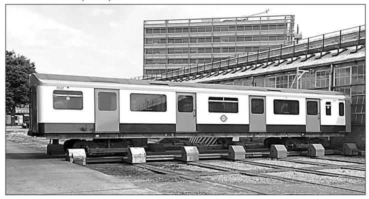
**Above:** D Stock DM 7027 on the traverser on 16 August 2016 before departure from Acton Works. Note that handles have been fitted to two single doors (on both sides), equipment has been removed from underside (although the motor bogies are) still attached, and that the car number has been moved from over the small window right next to the cab door. It is strange that the small section of white adjacent to the blue by each passenger door has been removed.
